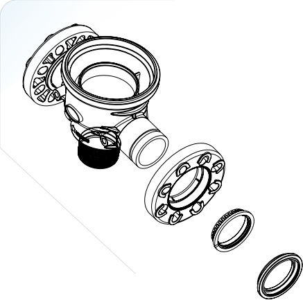
Connection Type: Victaulic/Threaded/Optionally 3" Flanged
