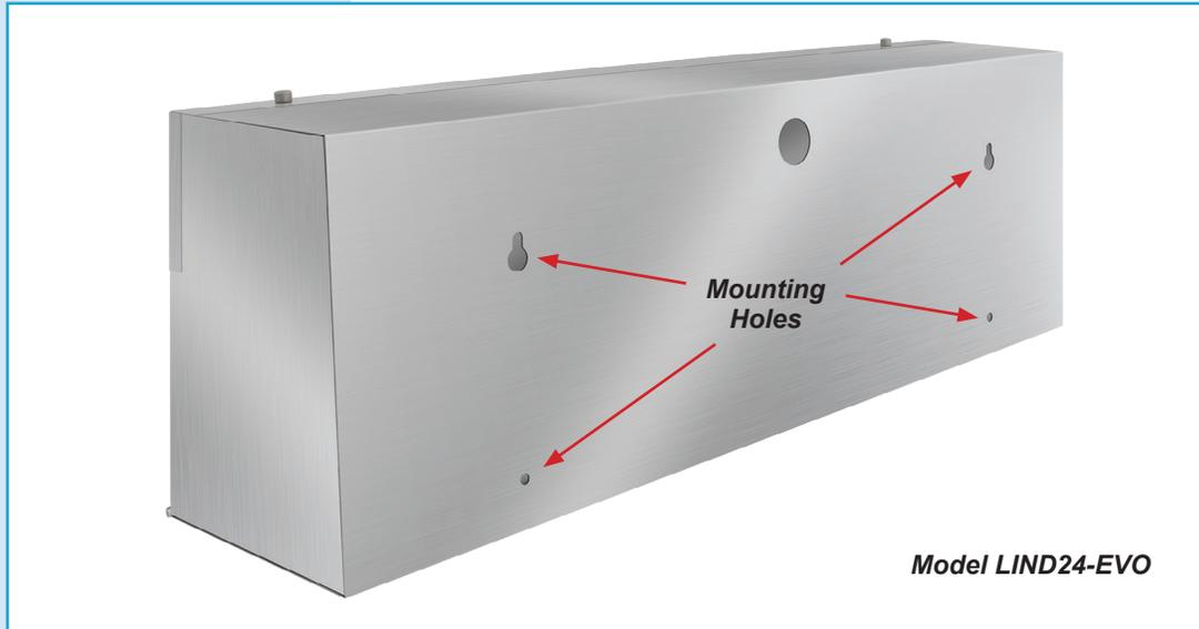
**Figure 1** – Shows the back side of **Hygeaire® Model LIND24-EVO**; note the four mounting holes in the back of the fixture. The fixture is to be mounted on a plumb and vertical surface, at a minimum height of 7 feet from the bottom of the fixture to the floor, in a location that must be able to safely support 16 pounds.
