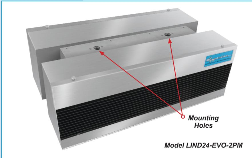
**Figure 2** – Shows the top of Hygeaire® Model LIND24-EVO-2PM (above). Note the two mounting holes on the top of this fixture (these are for the Pendant Mount Canopy Set attachment). The fixture is to be mounted at a minimum height of 7 feet from the bottom of the fixture to the floor, in a location that must be able to safely support 32 pounds.
