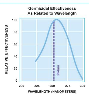
Approximately 95% of the ultraviolet energy emitted from **STER-L-RAY®** germicidal lamps is at 254 nanometers, the region of germicidal effectiveness most destructive to bacteria, mold, and viruses.
