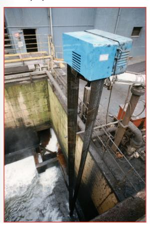
Abanaki provided Gregory with the **Grease Grabber**\*, a state-of-the-art skimmer that makes use of the differences in specific gravity and surface tension between oil and water. This allows the skimmer belt to attract grease, oil and other hydrocarbon liquids as the belt passes through the surface of the water, even under the most turbulent conditions.
