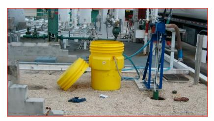
The **PetroXtractors**' simplicity was a great asset. After picking up the oil, the belts travel over head pulleys on each drive unit and through tandem wiper blades. Oil is then scraped off both sides of the belt and discharged through a small hose. Installation consists of merely lowering the belt and tail pulley into the casing until the pulley is fully immersed, placing the discharge hose in a container and switching the unit on.
