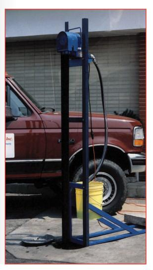
After weighing the advantages and disadvantages of passive methods and active pump systems, Chemviron selected a **PetroXtractor**® active belt skimmer from Abanaki Corporation, Chagrin Falls, Ohio.
