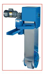
A unique part of the Abanaki oil skimmer operation is the ability of the head pulley to drive the belt without interfering with the oily residue on both sides of the belt. A free-riding tail pulley stabilizes belt operation but permits it to bend around floating obstructions that might damage permanently secured equipment.
